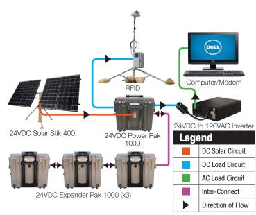
Figure 3 - Solar Stik RFID Power Solution
