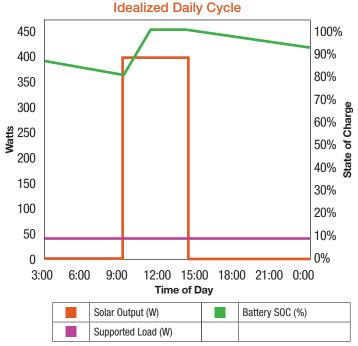
Figure 5 - Idealized daily cycle of RFID Solar Stik System
