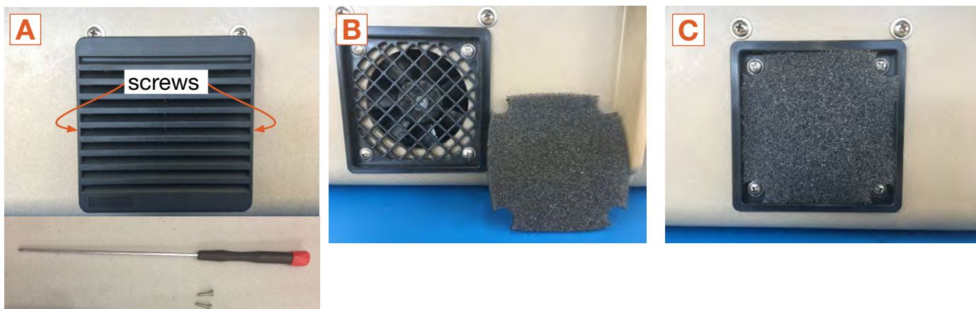
Figure 52. Cleaning the air intake filter
