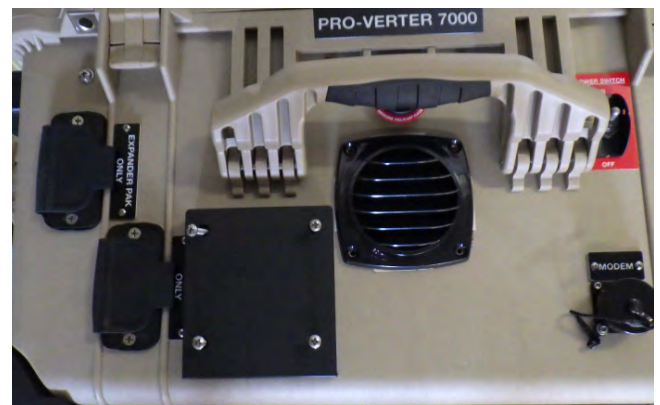
Figure 50. Removed vent shroud to access the louvered vent cover
