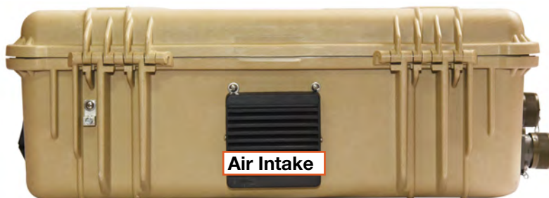
Figure 15. Power Hub rear side—Air intake vent
