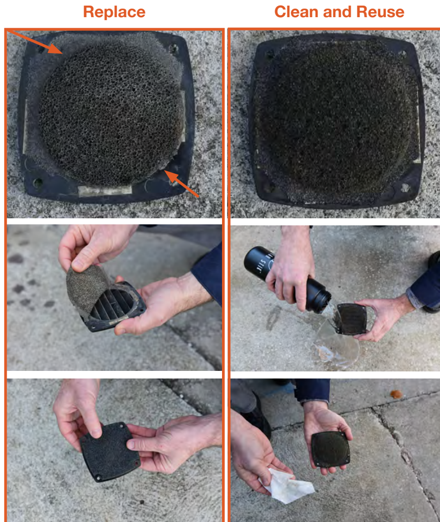
Figure 51. Replacing PRO-Verter filter (left); cleaning a PRO-Verter filter (right)
