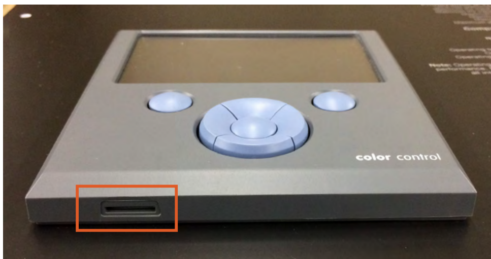
Figure 48. Micro SD card port location
