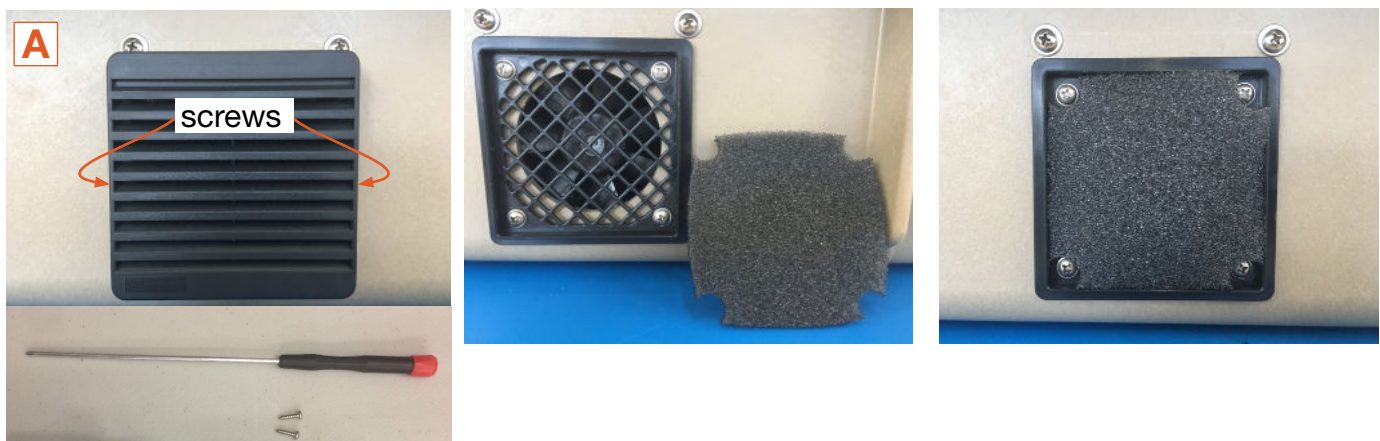
Figure 29. Cleaning the air intake filter
