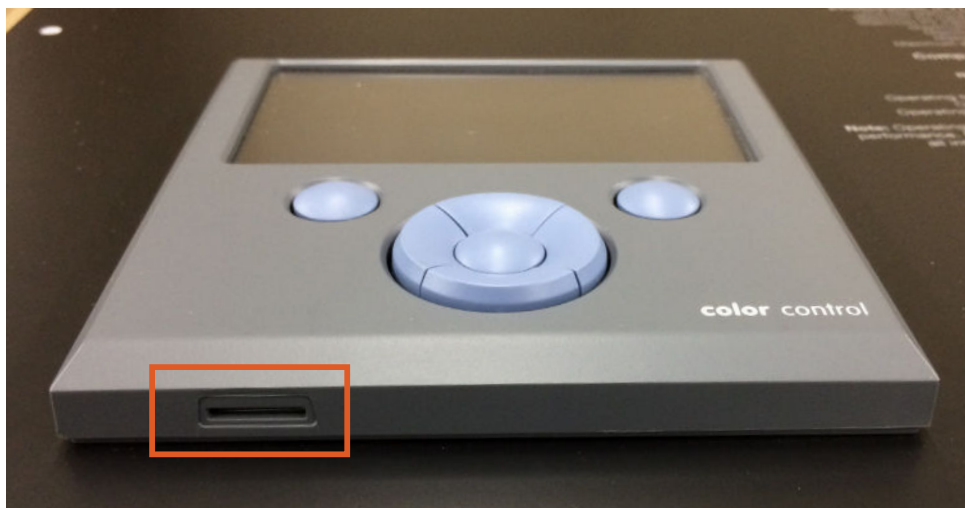
Figure 1. Micro SD card port location
