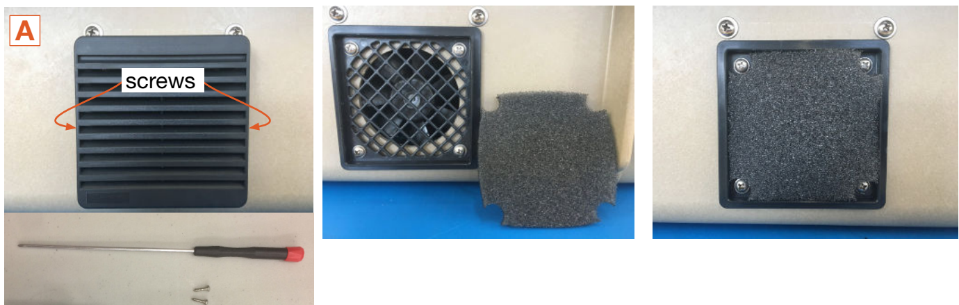
Figure 2. Cleaning the air intake filter
