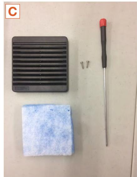
Figure 26. Removing the Power Hub air intake vent filter for cleaning
