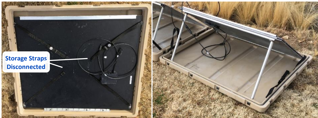
Figure 10. Un-stow Solar Panel Assemblies and lock the Solar Panel Support Tubes in
