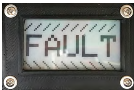
Figure 24. Battery Status Indicator - home page unattended fault warning
