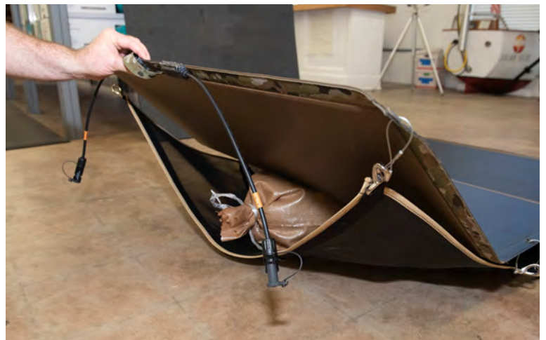
Figure 36. Sandbags placement for 0° deployment
