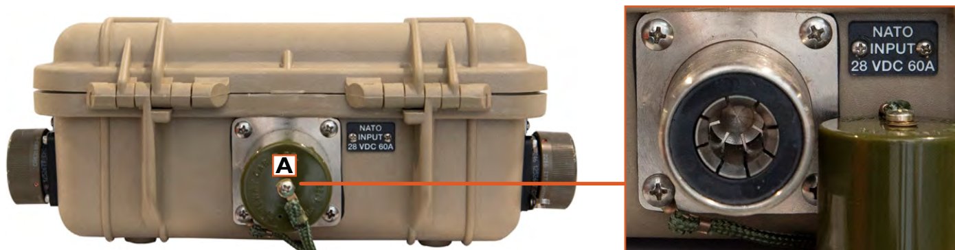
Figure 8. DC PDM NATO power input port
