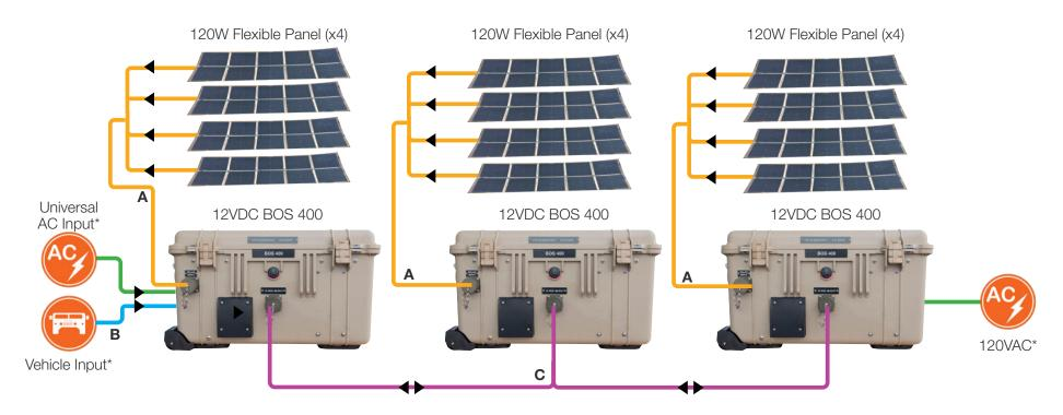
\*Universal AC Input, 9-36 VDC Input and 120 VAC Output are available on each BOS 400 unit.
