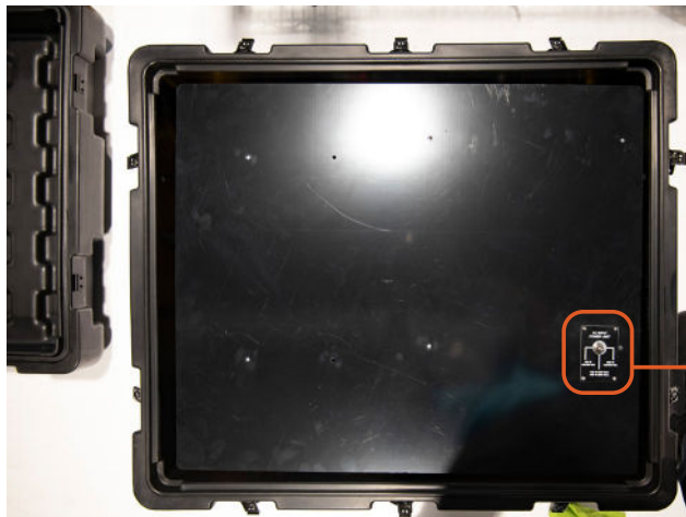
Top-down view of the AC Input Limit Switch located under the lid of the BOS.
