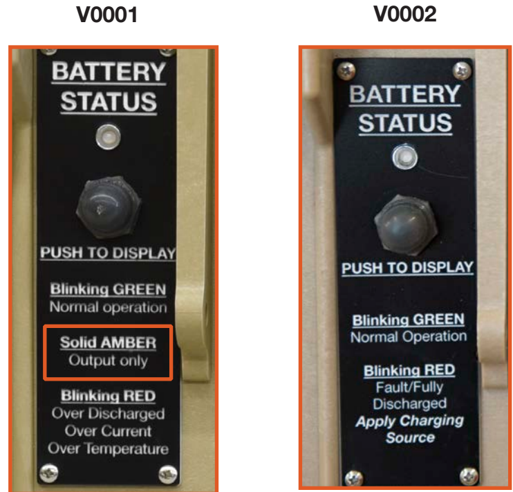
Figure 26. V0001 and V0002 Battery Status LED placards
