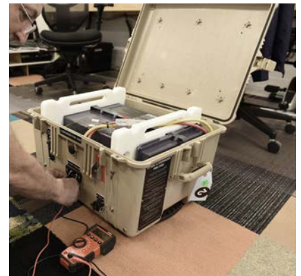
Figure 14. Measuring voltage across terminals of Inter-Connect port
