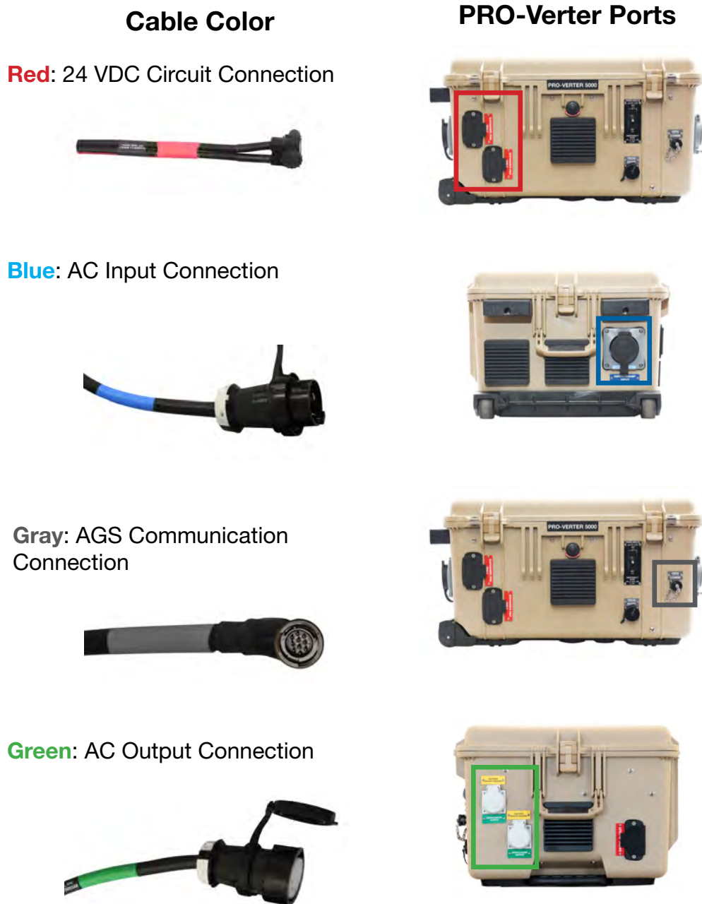
Figure 8. System connection color coding
