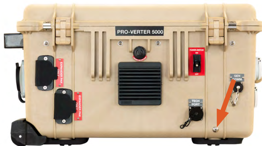
Figure 23. Location of drain plug screws in the PRO-Verter 5000
