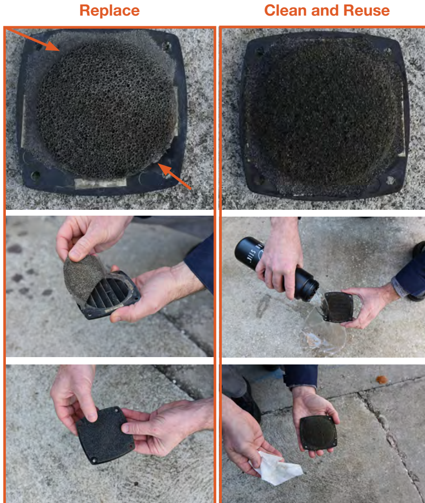
Figure 33. Replacing PRO-Verter filter (left); cleaning a PRO-Verter filter (right)
