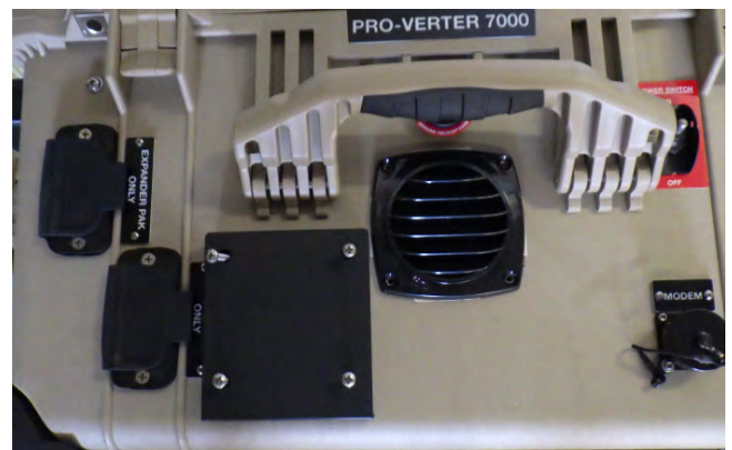
Figure 32. Removed vent shroud to access the louvered vent cover
