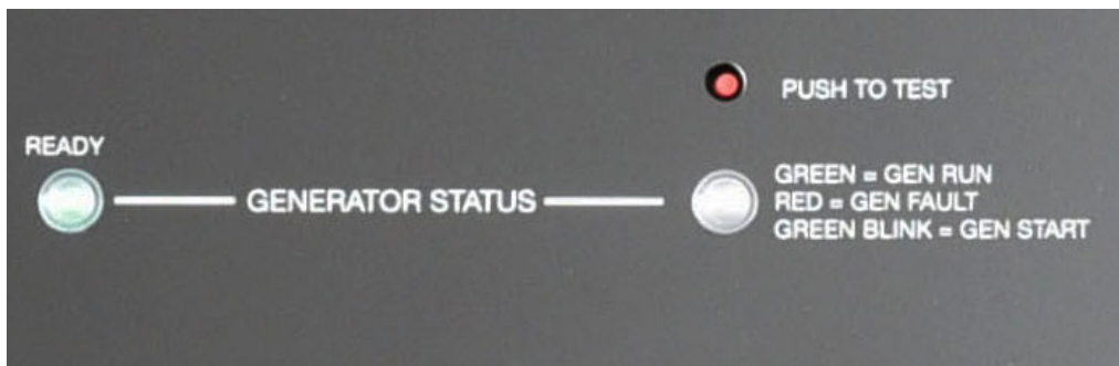
Figure 17. Generator Status LEDs
