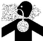
Never operate the generator in an enclosed area. Operating a generator indoors can kill you in minutes. Generator exhaust contains carbon monoxide. This is a poison you cannot see or smell. Only operate the generator outside and far away from windows, doors and vents.
