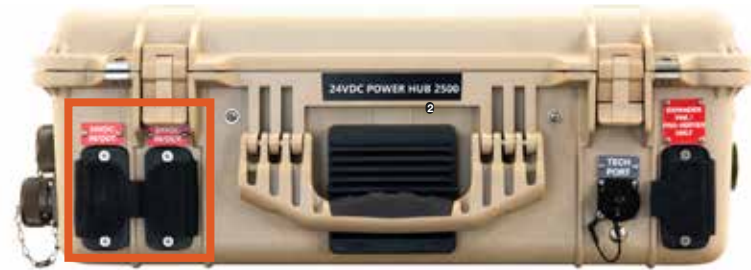
Figure 15. Power Hub 24 VDC IN/OUT ports
