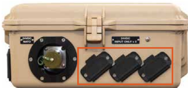
Figure 13. Power Hub regulated 24 VDC inputs
