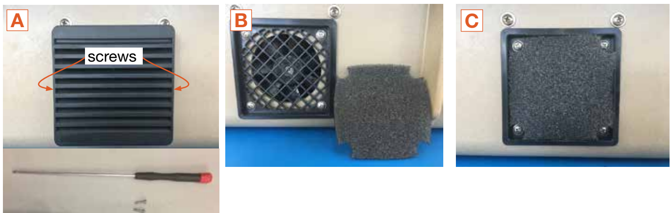
Figure 29. Cleaning the air intake filter
