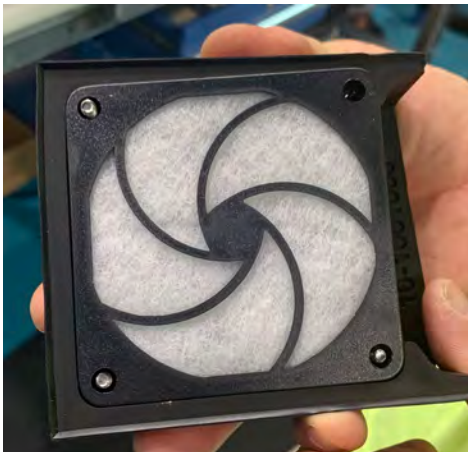
Figure 27. Proper orientation of replacement filter cassette.
