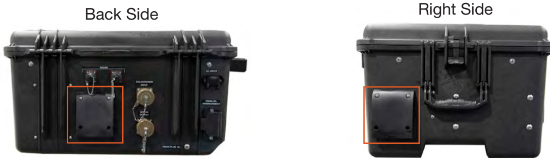
Figure 26. Replacing (or cleaning) the PGA Power Module air filters
