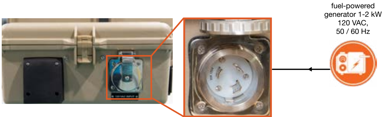
Figure 15. Connecting generators to HyPR
