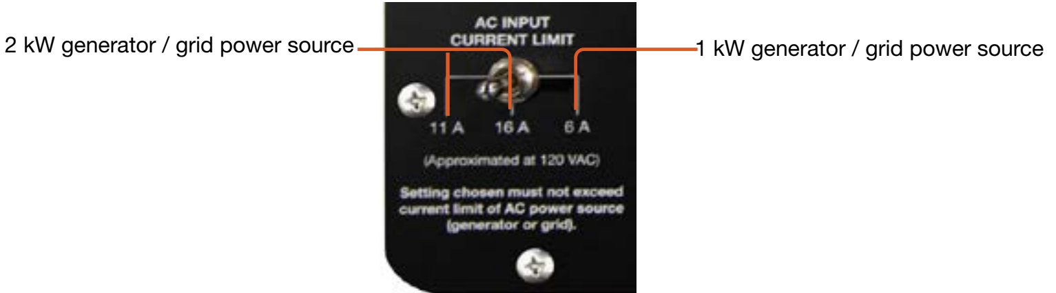
Figure 13. AC Input Current Limit Switch
