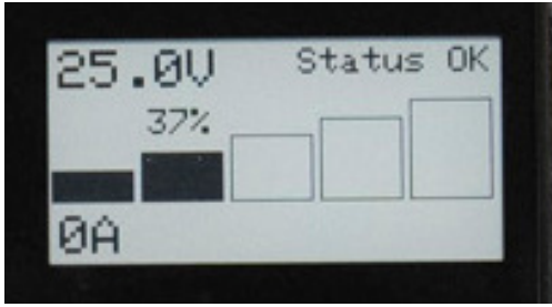
Figure 16. Battery Status Indicator home page “dead battery”
