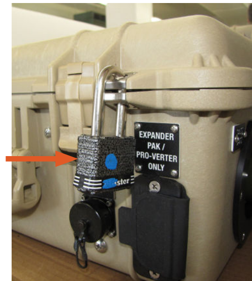
Figure 26. Lock securing Power Hub lid
