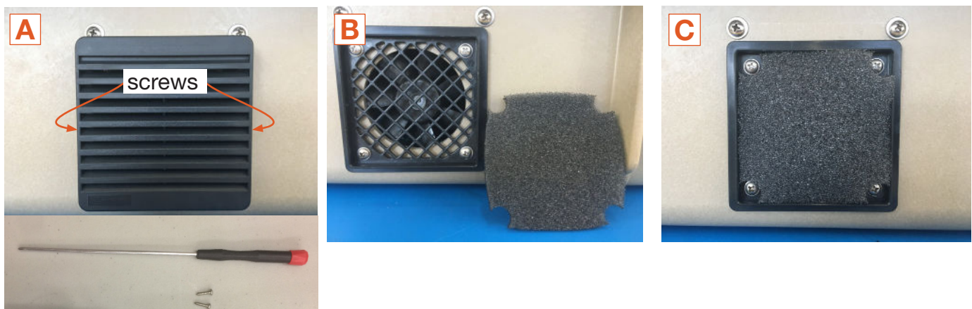
Figure 29. Cleaning the air intake filter
