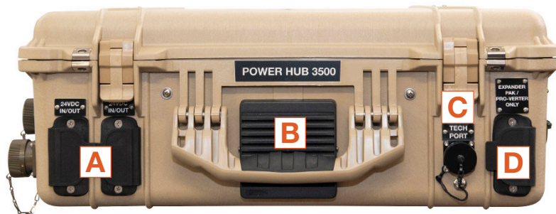
Figure 6. Front—DC output and communications
