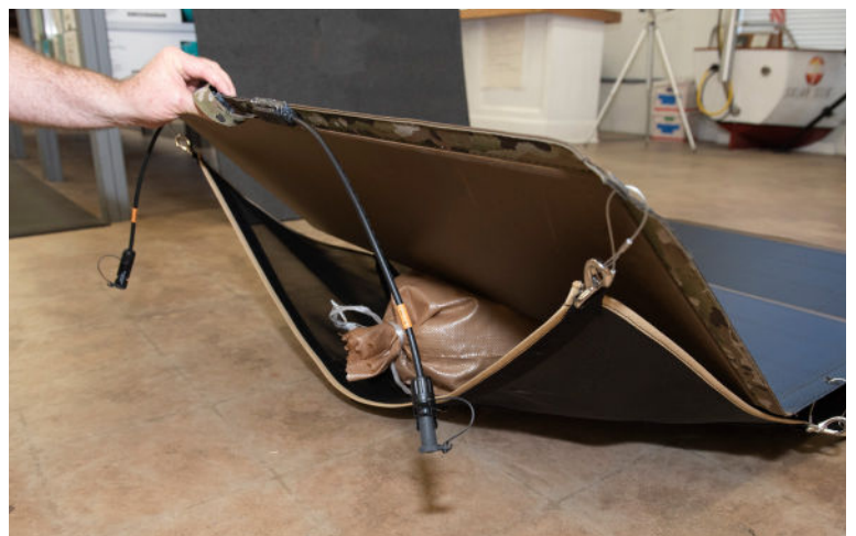
Figure 10. Sandbags placement for 0° deployment
