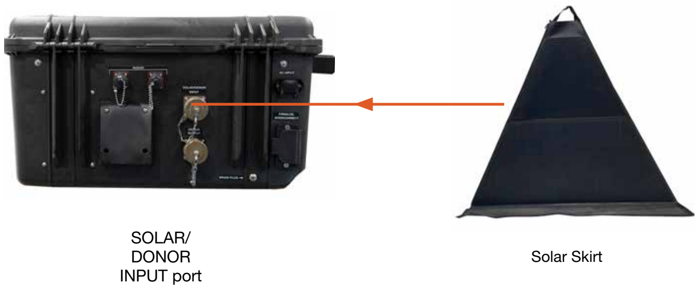
Figure 7. Connecting the Solar Skirt to the Power Module
