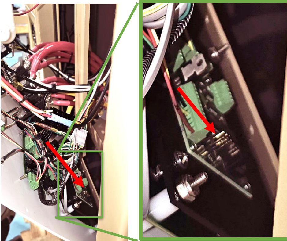
Figure 2 - view of open faceplate from the right side of the faceplate, arrow indicates 2x3 header
