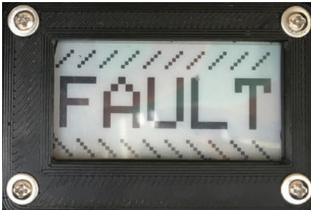
Figure 6. Battery Status Indicator - home page unattended fault warning
