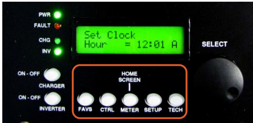
Figure 16. Menu buttons on the LCD User Interface
