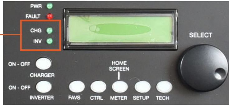
Figure 5. Invert and charge mode LEDs on User Interface
