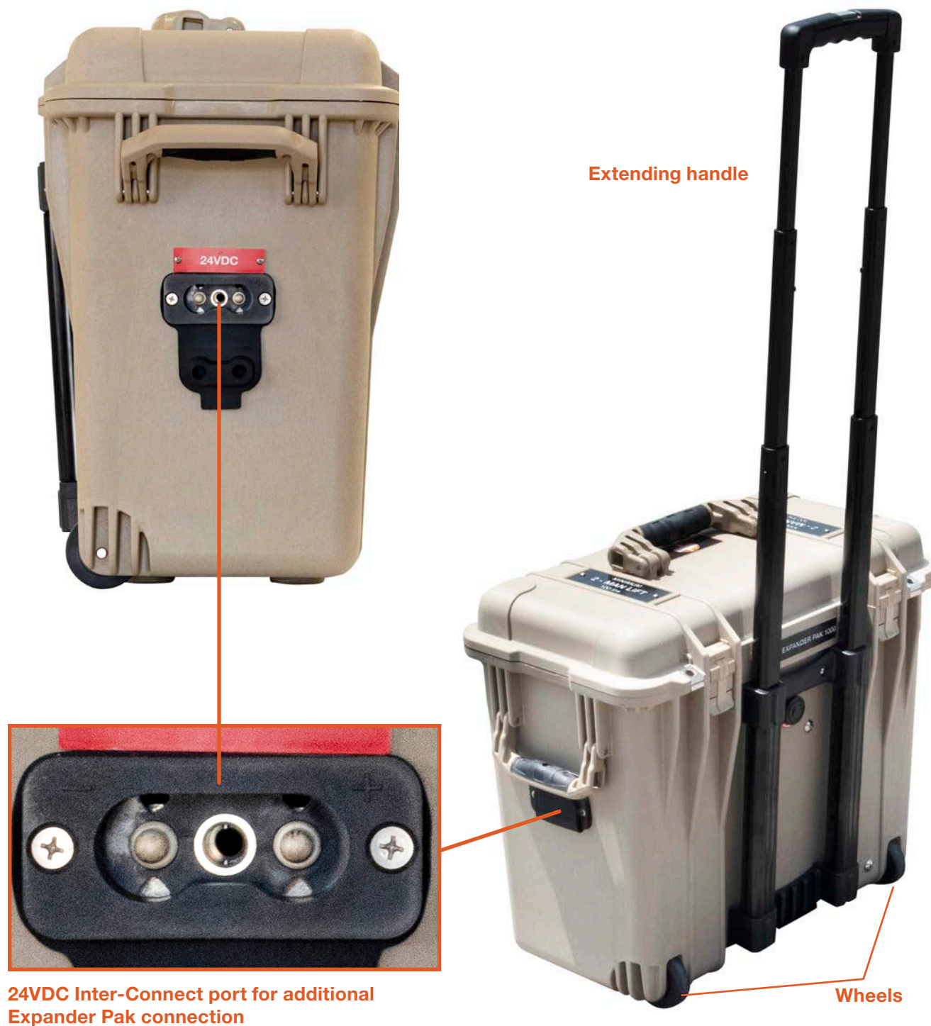
Figure 5. Expander Pak 1000 exterior views and descriptions
