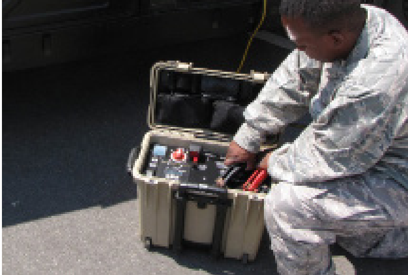
Figure 8. Recharging from a vehicle’s 24-volt system
