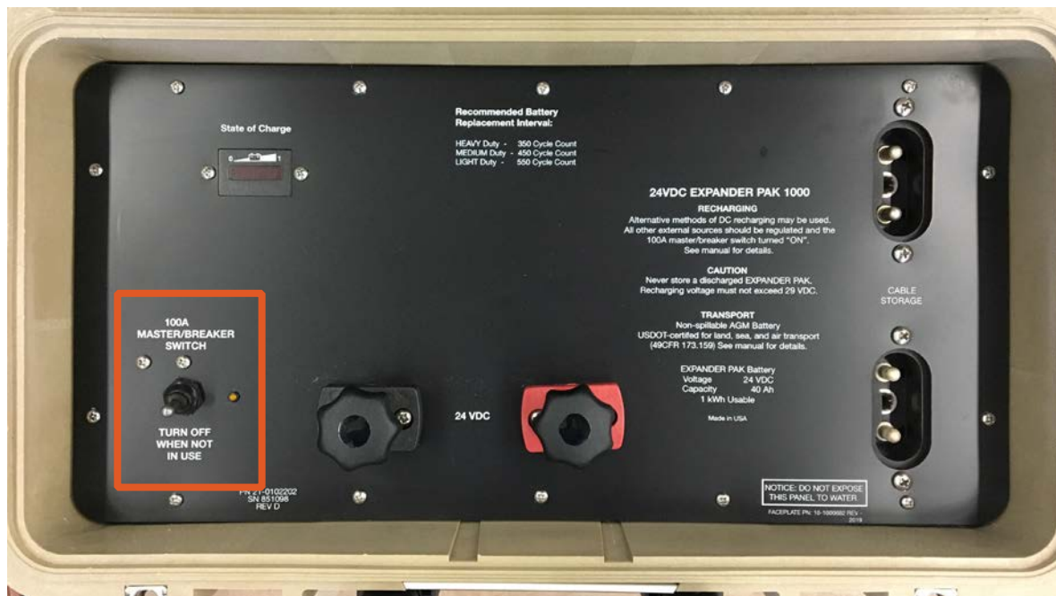
Figure 6. 100 A master breaker switch and indicator LED
