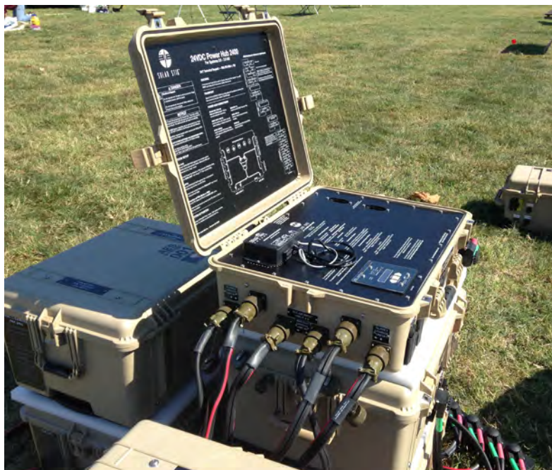
Figure 1. A Power Hub in a Hybrid Power System
