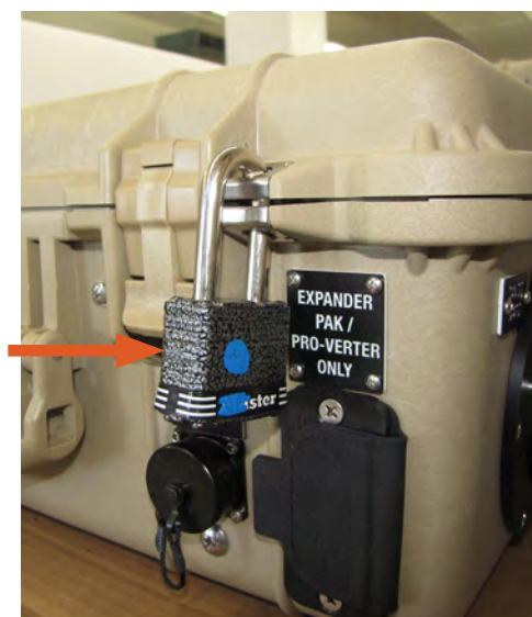
Figure 26. Lock securing Power Hub lid
