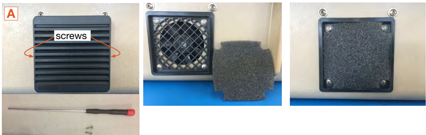
Figure 29. Cleaning the air intake filter
