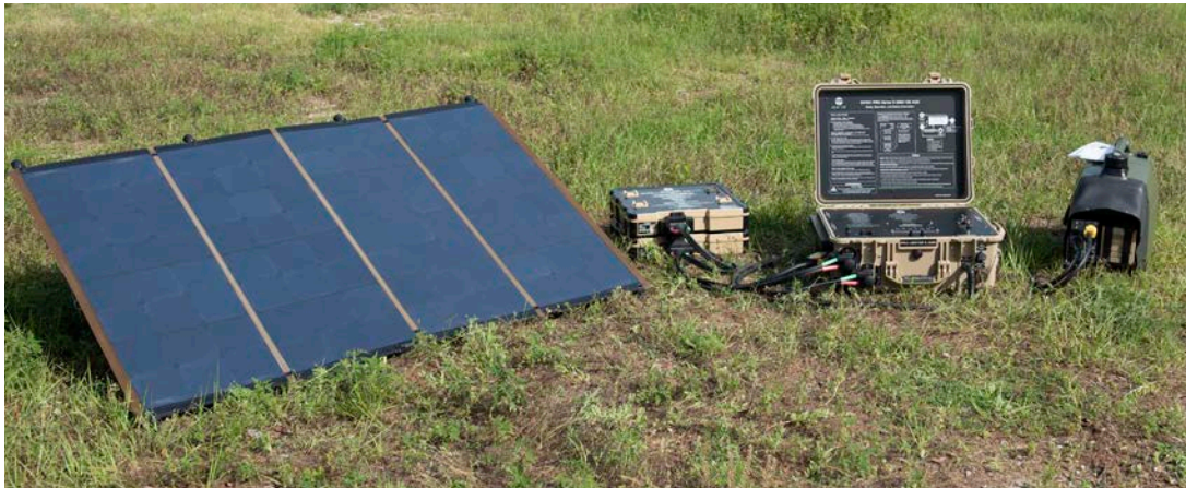
Figure 2. Solar Venture 350W four-panel PV array with a small HPS
