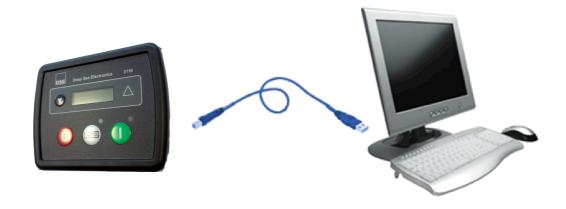
ANOTE:- The DC supply must be connected to the module for configuration by PC.
