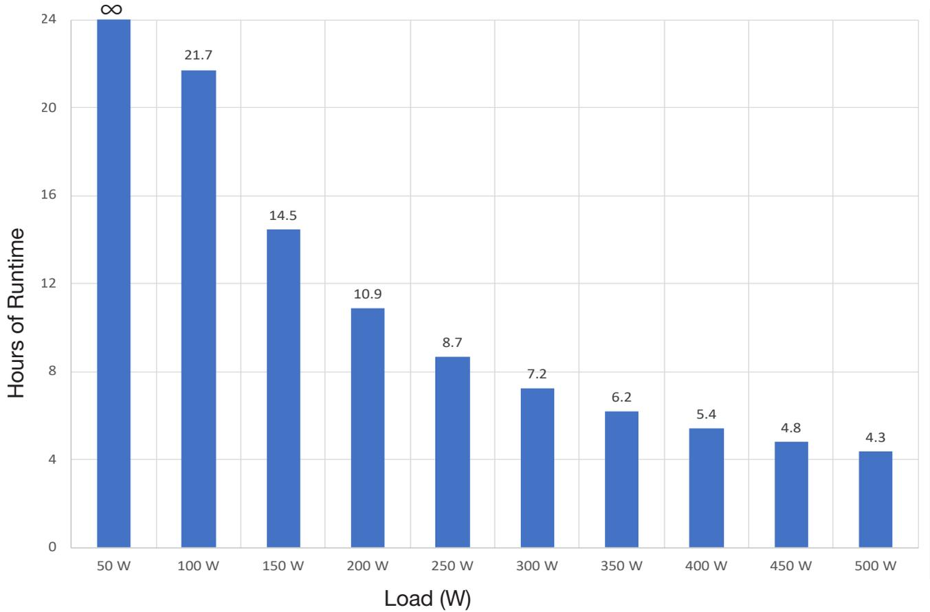
Figure 28. System runtime at various loads with PV power only
