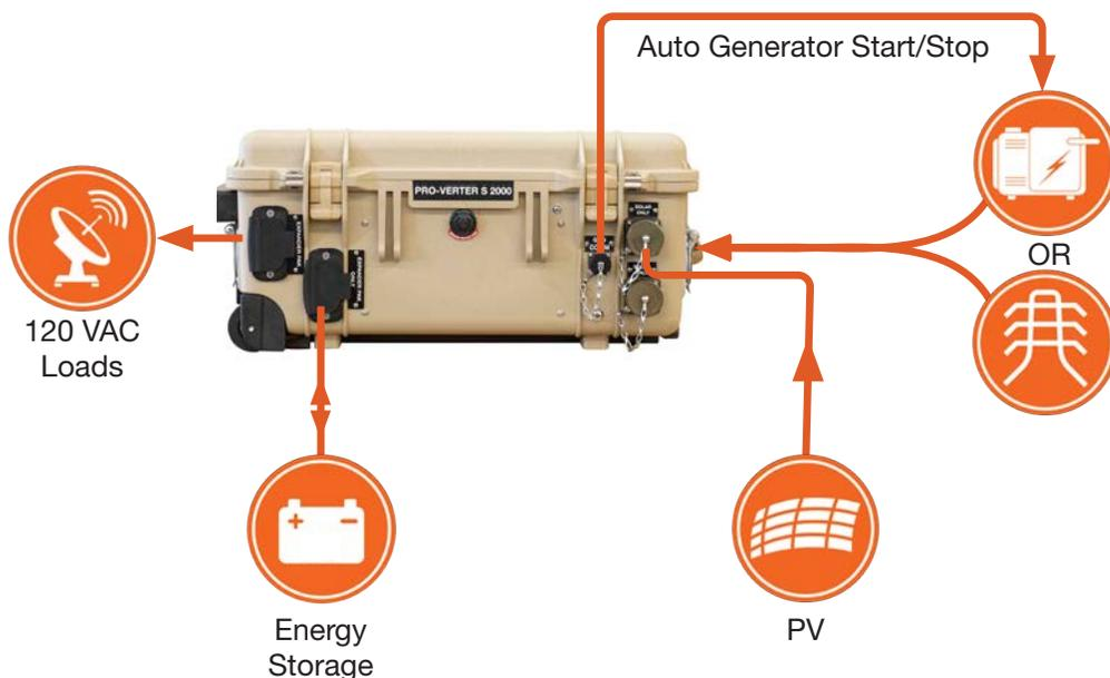
Figure 2. PRO-Verter S 2000 circuits
