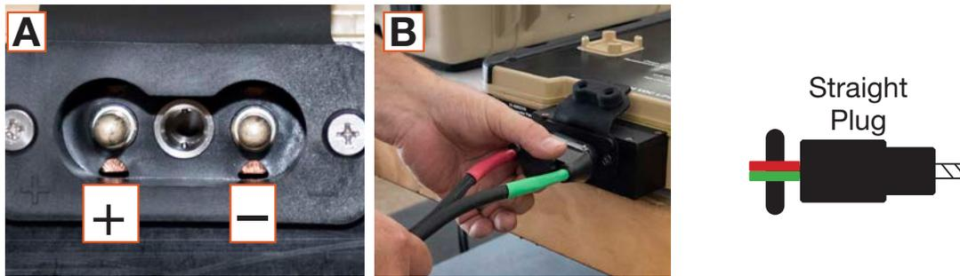
3. Connect the “angled” Inter-Connect plug to the Inter-Connect Strip 7. Use a standard Inter-Connect cable with two (2) angled ends to connect the Inter-Connect Strip to the PRO-Verter Expander Pak only Inter-Connect port.
