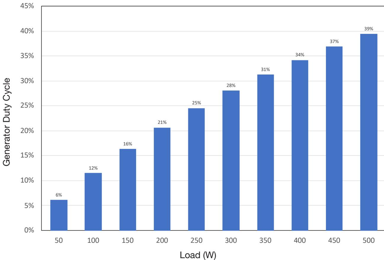
Figure 27. 1 kW generator duty cycle as a function of continuous loads.
