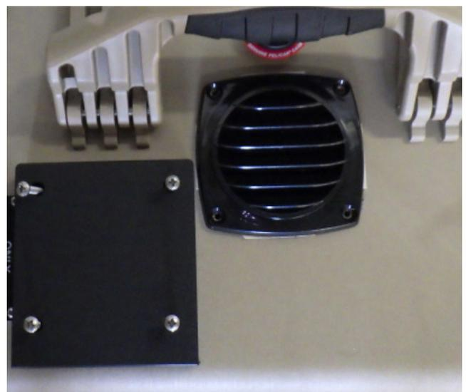
Figure 32. Removed vent shroud to access the louvered vent cover
