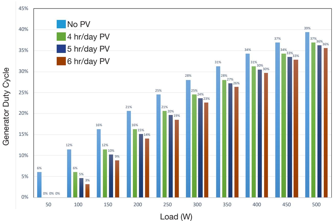
Figure 29. Increasing PV power input reduces generator duty cycle.
