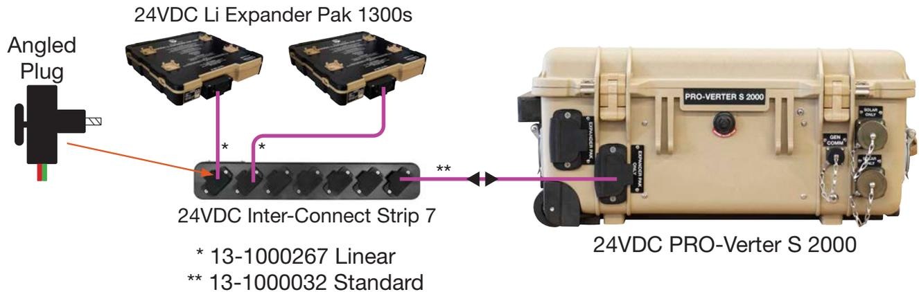
Figure 15. PRO-Verter to ESM connection
