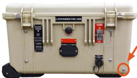
Figure 21. Li Expander Pak drain plug location
