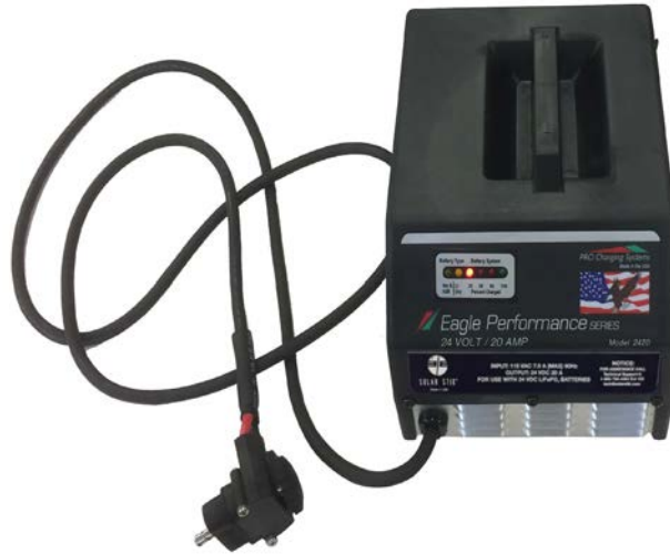
Figure 12. 24VDC Li Battery Maintainer with Inter-Connect Plug
