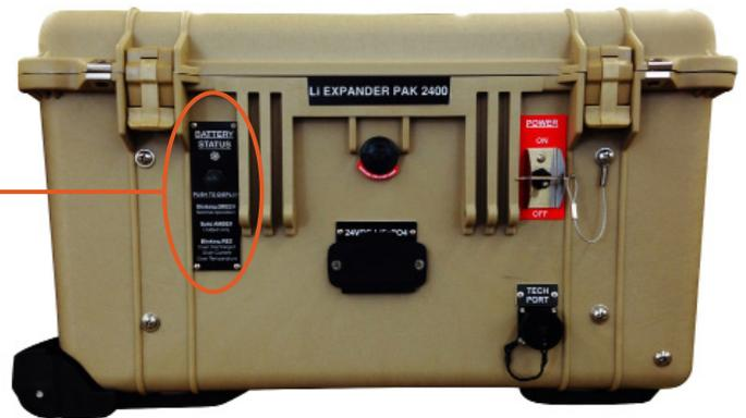
The Status LED provides information about the operational and error modes of the Li Expander Pak 2400. The meanings are in the table below.
