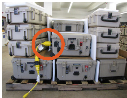
Figure 5 - Adaptor Cables attached to the AC input connection on the PRO-Verter 7000
