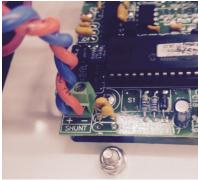
**B**. Trace the wires to the shunt block (arrow) on the interior wall of the component
