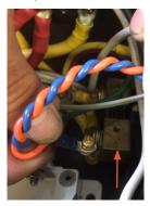
**C**. Remove both of the screws that hold the wires to the shunt block.
