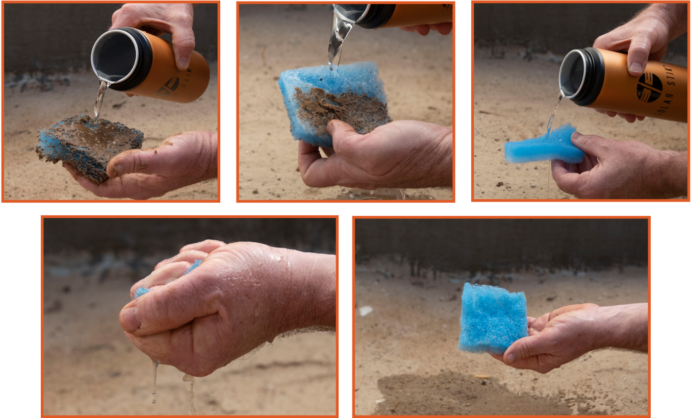
Figure 4. Washing the Power Hub filter
