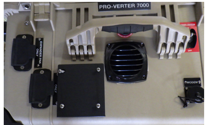
Figure 11. Removed vent shroud to access the louvered vent cover
