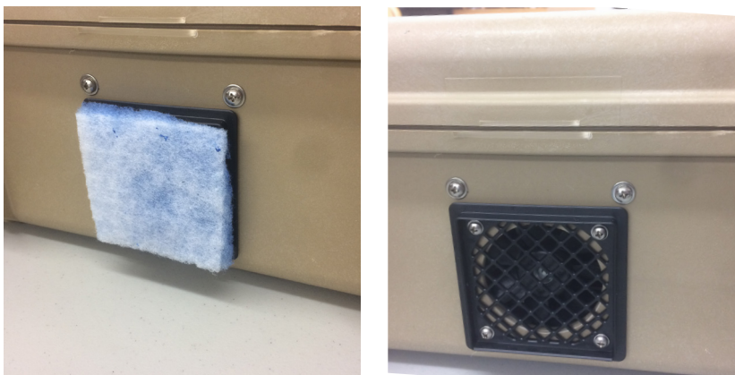
Figure 3. Exposed filter and vent
