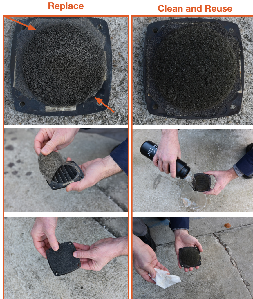
Figure 12. Replacing PRO-Verter filter (left); cleaning a PRO-Verter filter (right)
