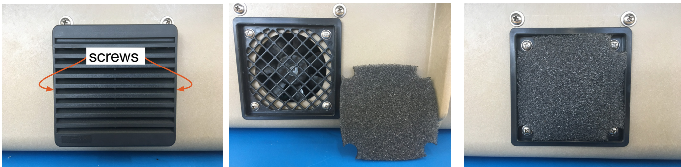
Figure 5. Installation of updated air intake vent filter material
