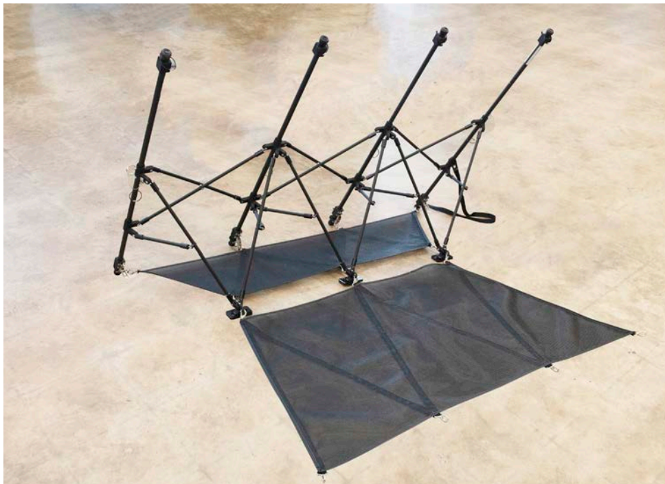
Figure 9. Ground-securing mesh configuration for 60° array deployment
