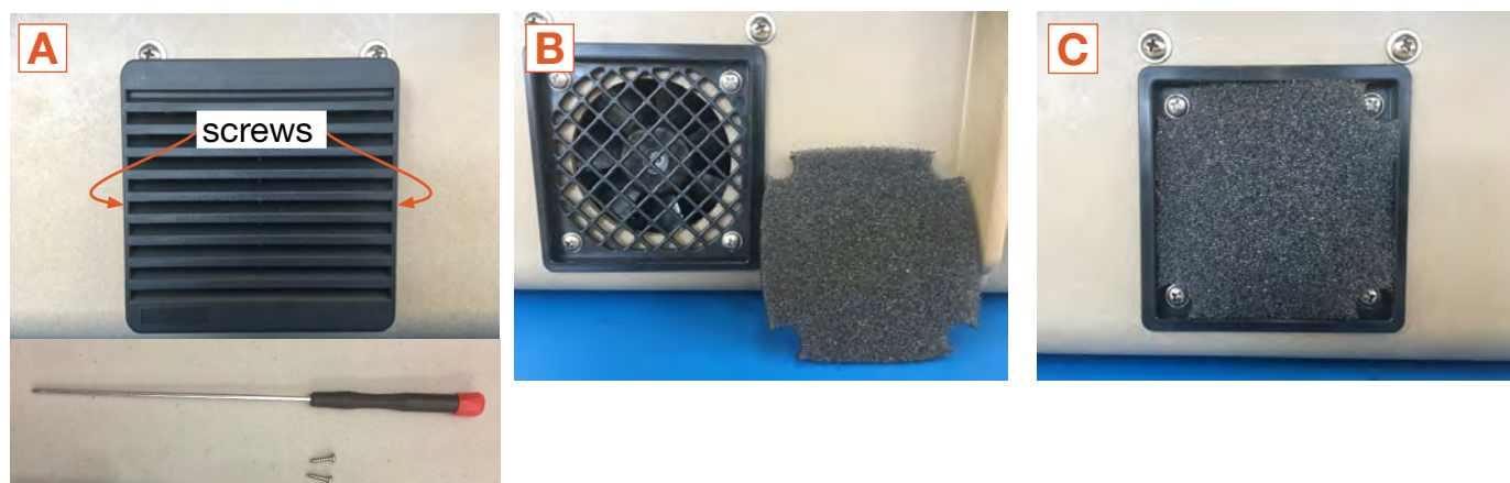
Figure 52. Cleaning the air intake filter
