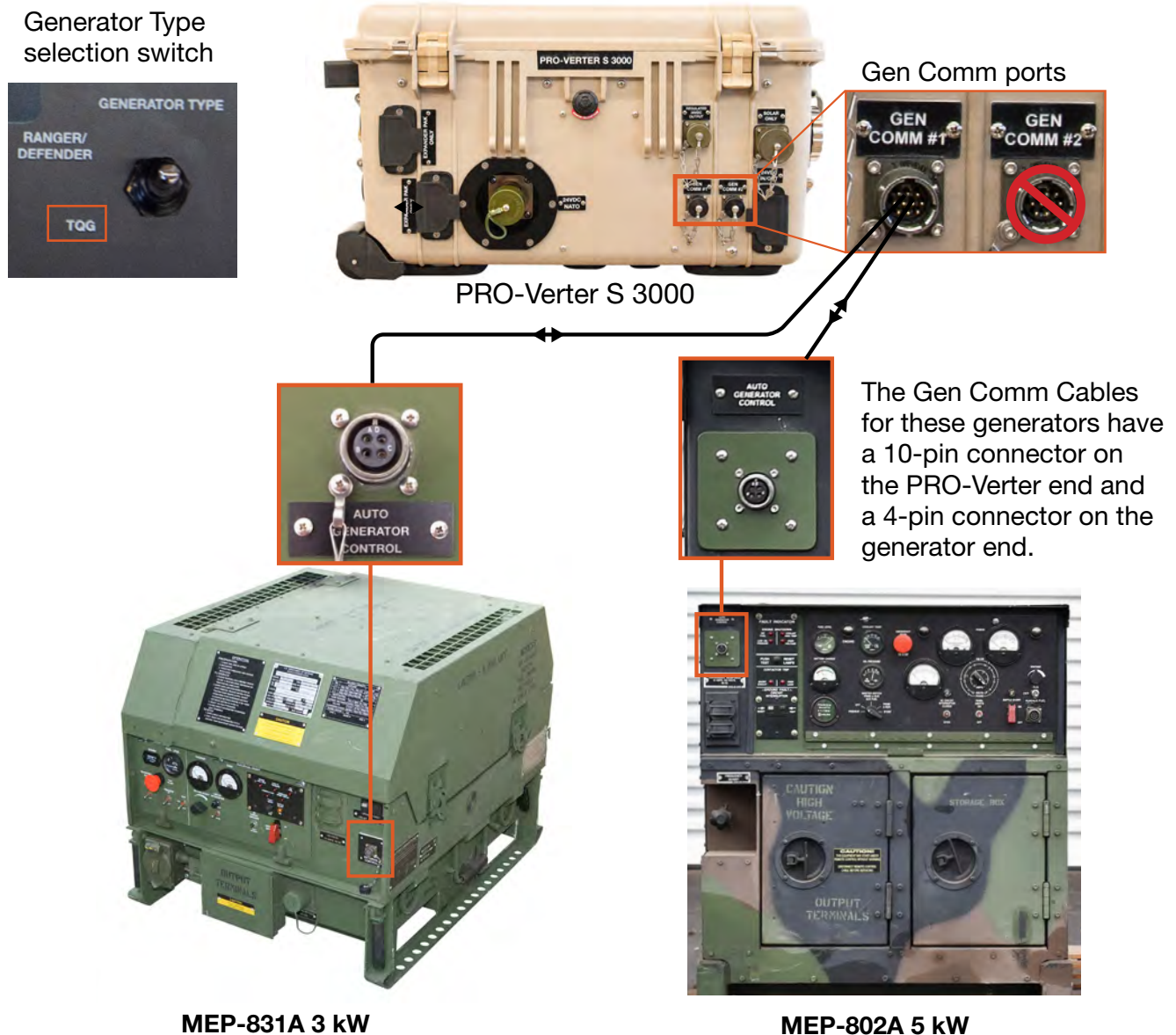
Figure 29. MEP-831A and MEP-802A Gen Comm Cable connections
