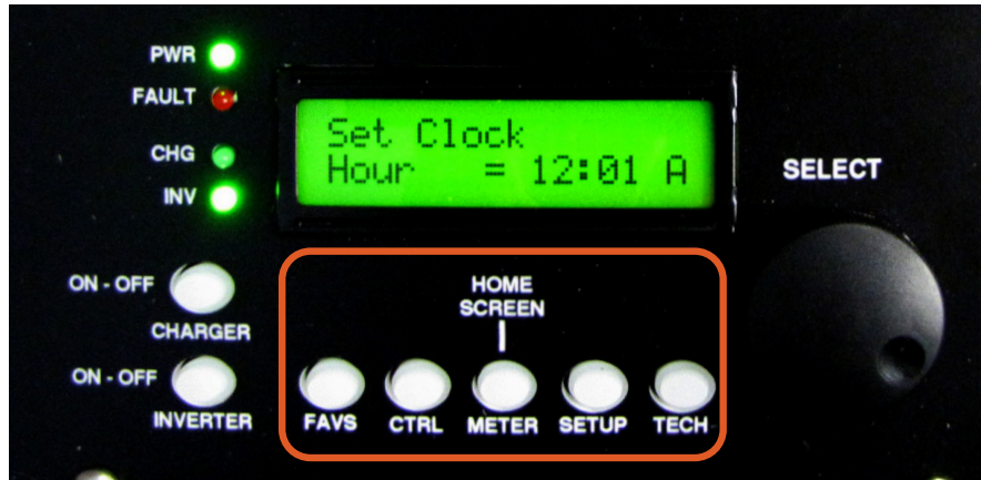
Figure 20. Menu buttons on the LCD user interface
