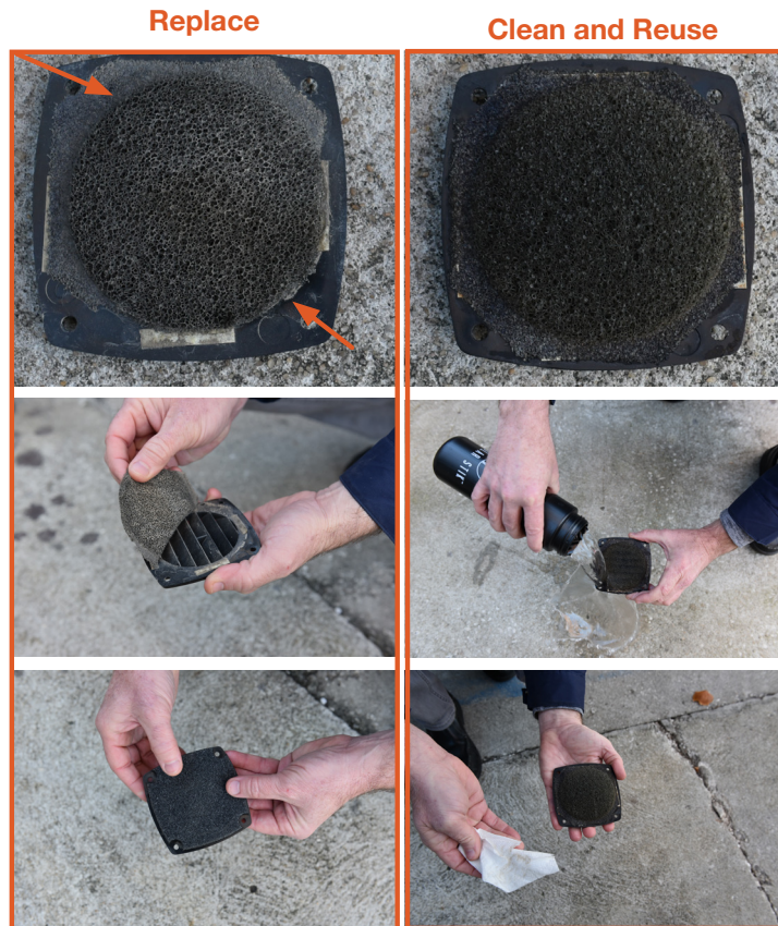
Figure 23. Replacing PRO-Verter filter (left); cleaning a PRO-Verter filter (right)
