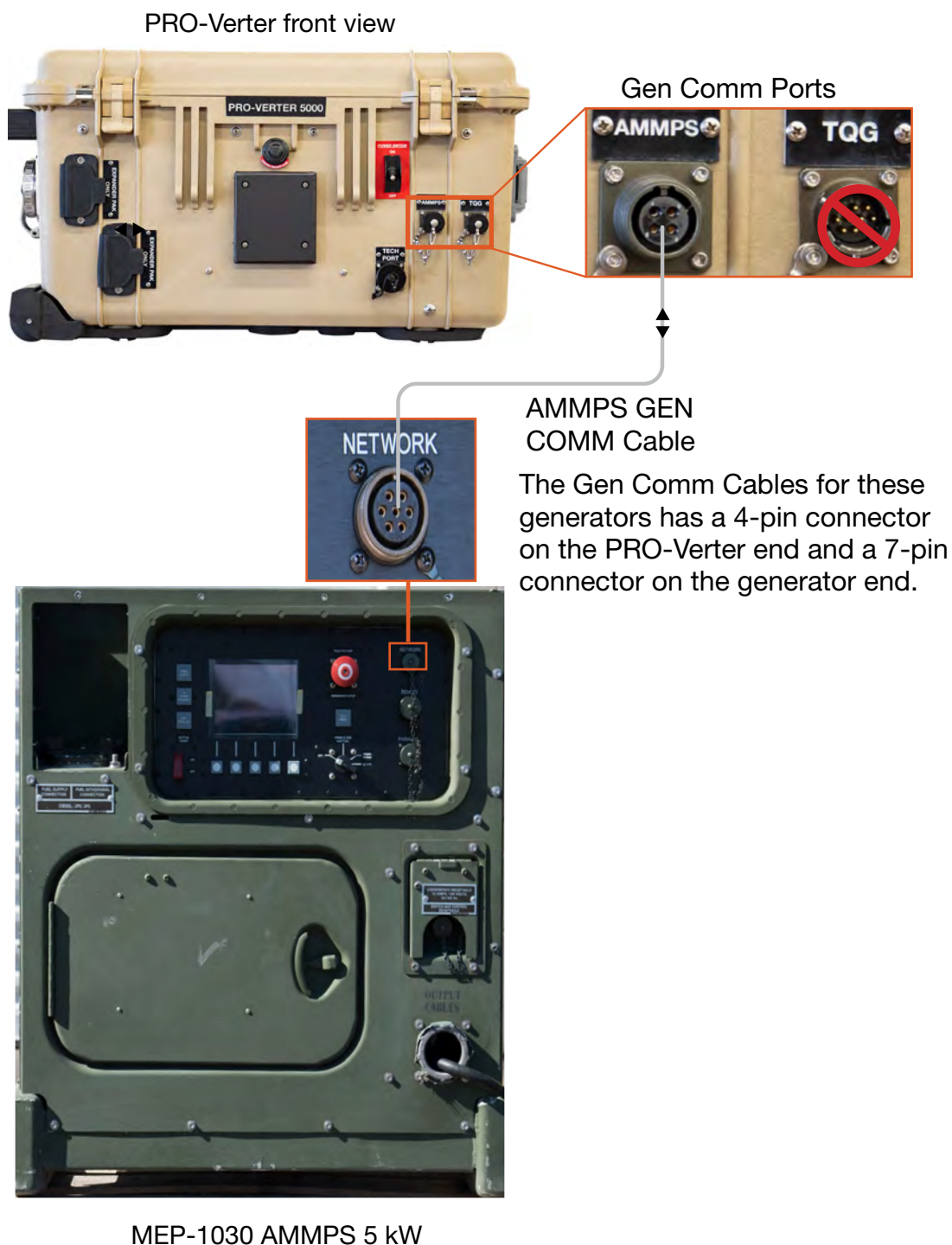
Figure 21. MEP-1030 AMMPS 5 kW Generator Communication Cable connections
