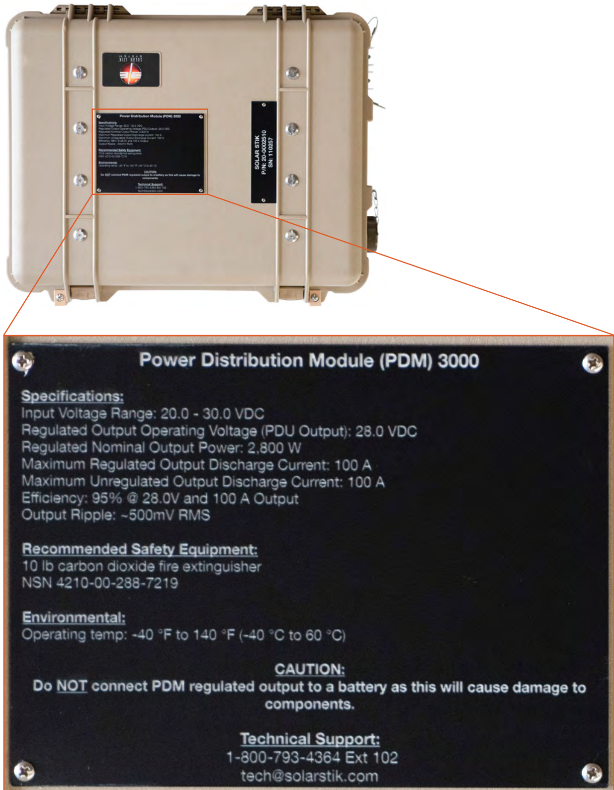
Figure 11. PDM 3000 top, Faceplate, specs, and cautions
