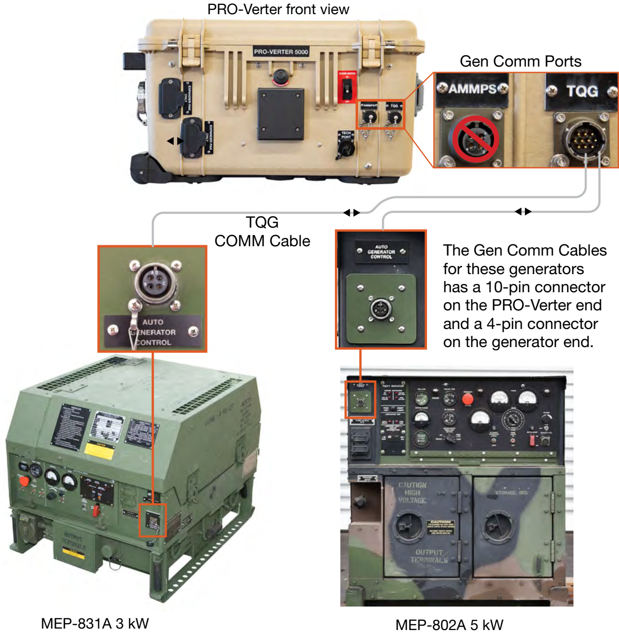
Figure 20. MEP-831A and MEP-802A Generator Communication Cable connections
