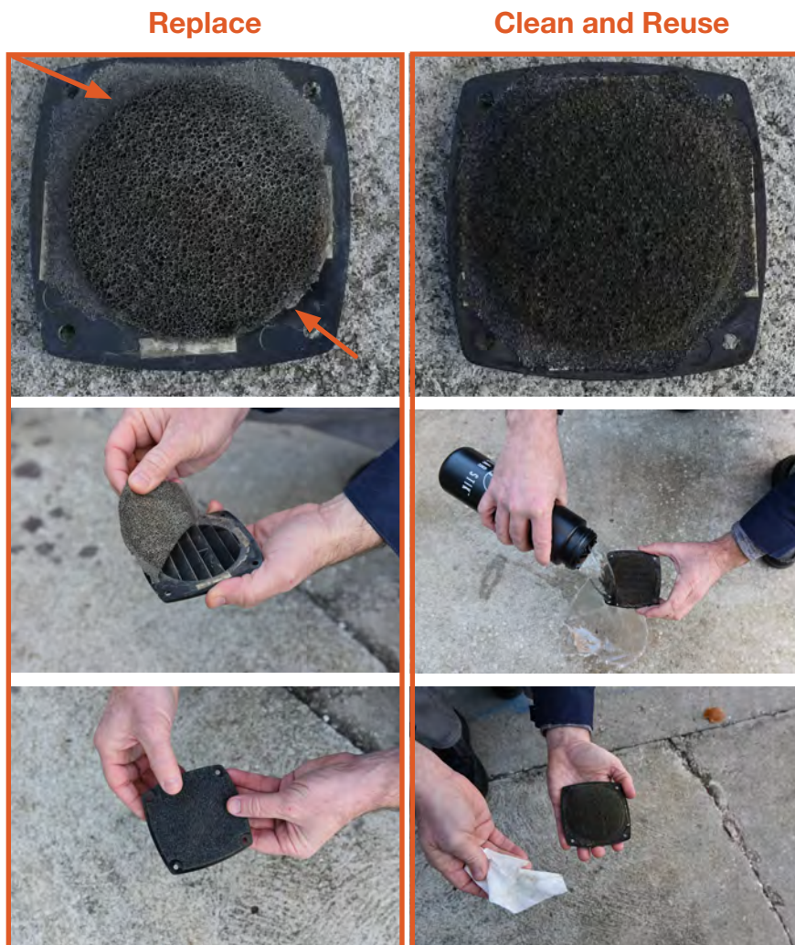
Figure 28. Replacing PRO-Verter filter (left); cleaning a PRO-Verter filter (right)
