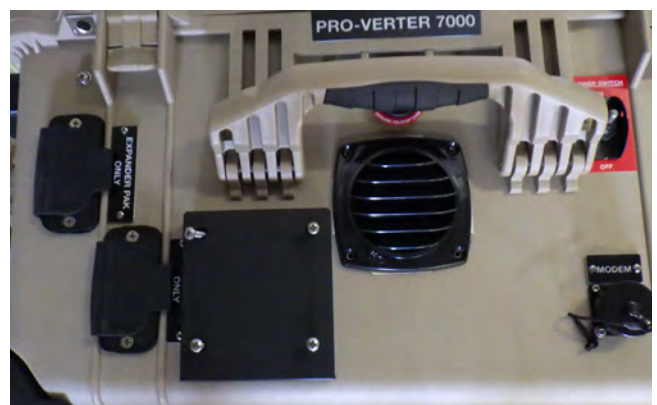
Figure 27. Removed vent shroud to access the louvered vent cover
