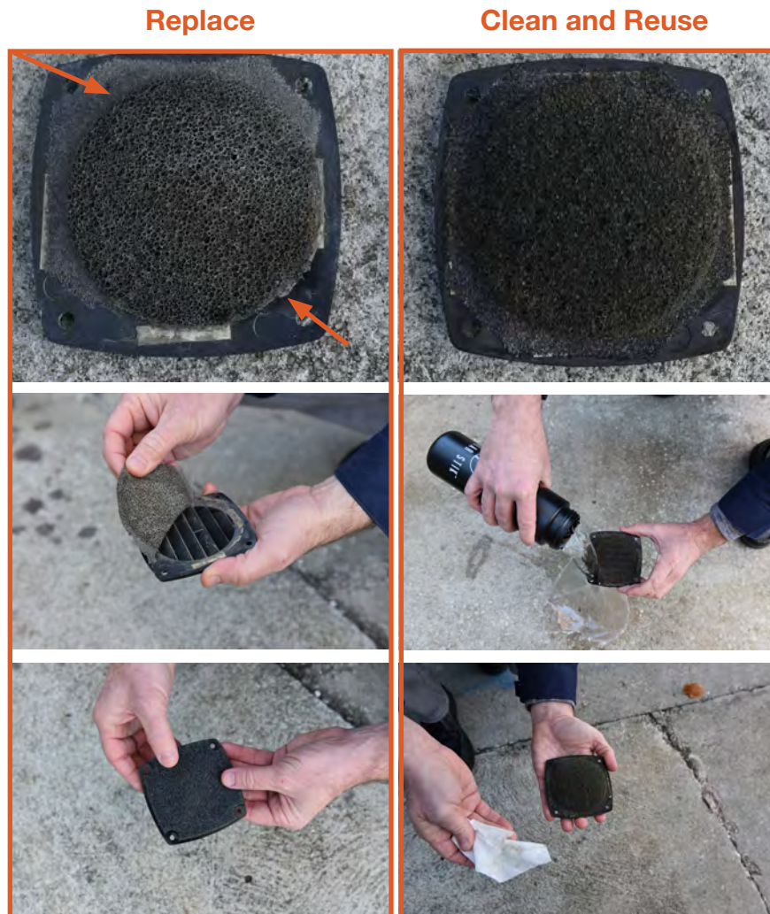
Figure 34. Replacing PRO-Verter filter (left); cleaning a PRO-Verter filter (right)
