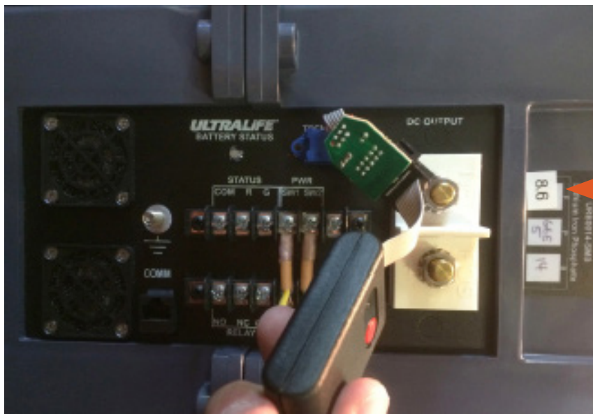
Figure 31. Firmware Loader connected to the MKM Tech Port
