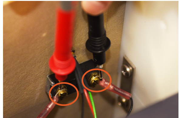
Figure 19. Momentary switch fasteners
