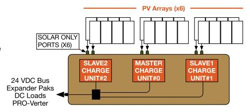
Figure 30. Power Hub 2400 SOLAR INPUT ONLY ports and their connection to charge controllers
