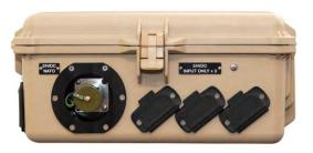
Connect regulated 24 VDC power sources such as wind generators and fuel cells to the three (3) Inter-Connect ports. Connect 24 VDC power from Military Vehicles (e.g., HMMWV) and TQGs to the NATO port.
