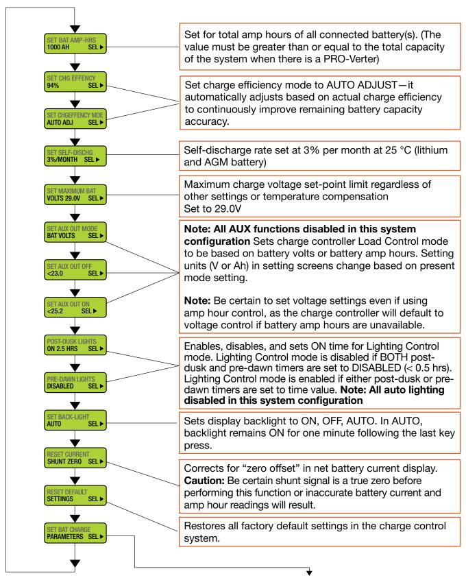
**To Battery Charge Parameter Setup Menus**
