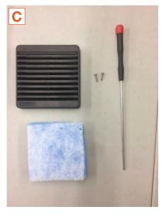
Figure 26. Removing the Power Hub air intake vent filter for cleaning
