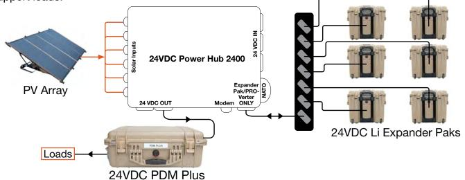
Figure 28. Power Hub as the primary power management device
