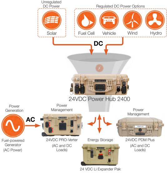
Figure 2. How a Power Hub works in a System
