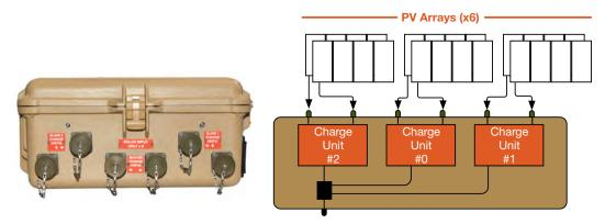
Figure 13. Power Hub Solar Input Only connectors
