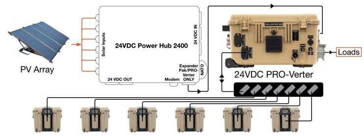
Figure 29. Power Hub as the secondary power management device
