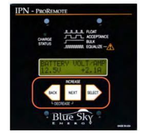
• To change settings / parameters in the SETUP and BATTERY CHARGE PARAMETERS menus, move forward through the menus (using the steps above) to the referre window that contains the thors desired parameter. Then do the following:
