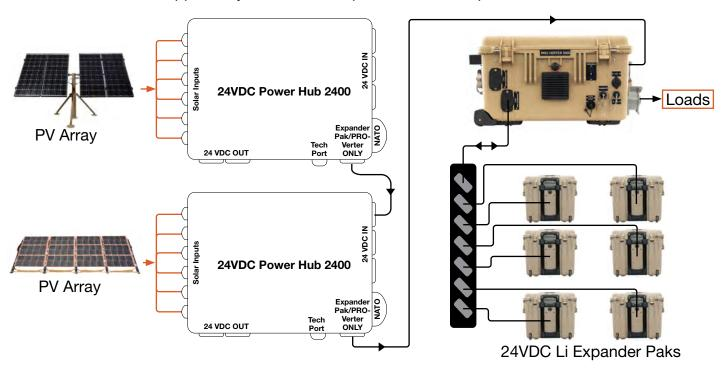
Figure 27. Stacking Power Hubs
