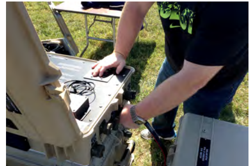
Figure 13. Connecting Solar Arrays to a Power Pak or Power Hub solar-only port
