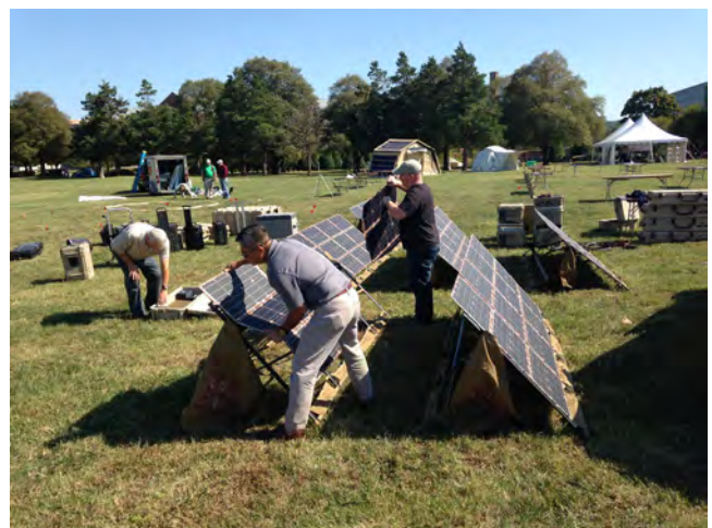
Figure 5. Setting up the Expedition Solar Array-C
