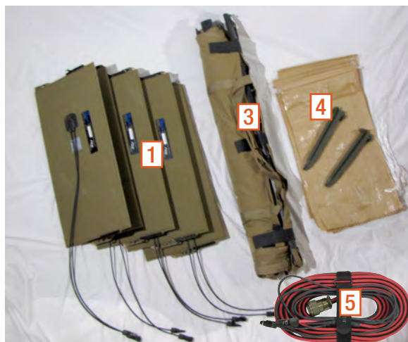
Figure 2. 420W Expedition Solar Array-C components in transport case (top) and unpacked (bottom)
